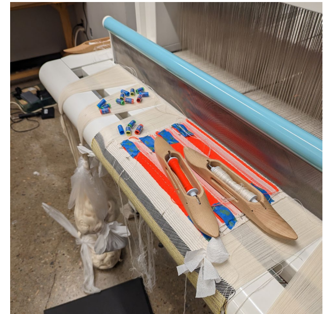
The work in progress on a TC2 Jacquard loom. Hand-wound coils and magnets are woven into complex weave structures in multiple layers of the cloth.
